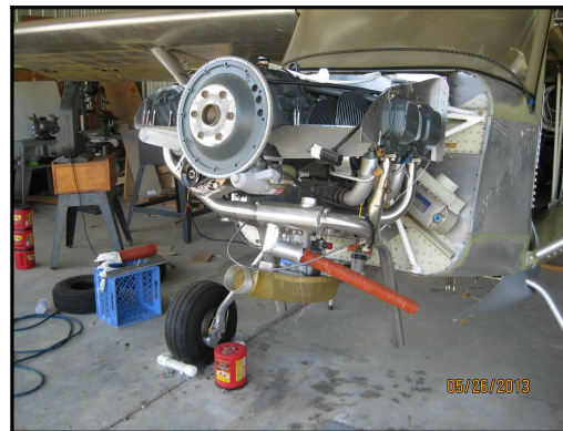
Fresh, zero time 180 hp. engine
